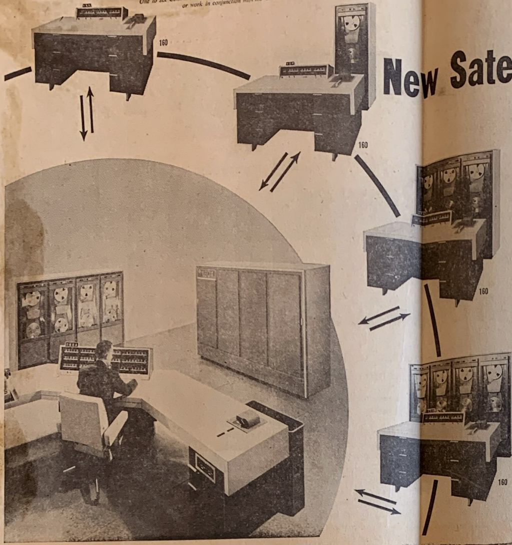
One to six Control Data 160 Computers act as independent "satellite" data processing centers, or work in conjunction with the Control Data 1604 Computer.
